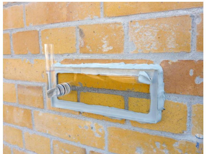
Figure 3. Testing panel for water permeability as per Prof. Franke is used on a historical fair-faced masonry façade.
