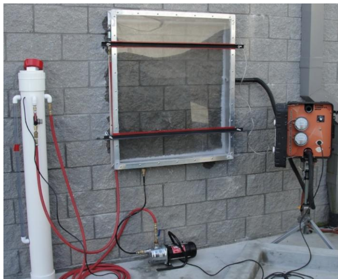
Figure 4. Measuring instrument determination of water absorption of masonry facades after ASTM C1601 (BDG-USA 2015).
