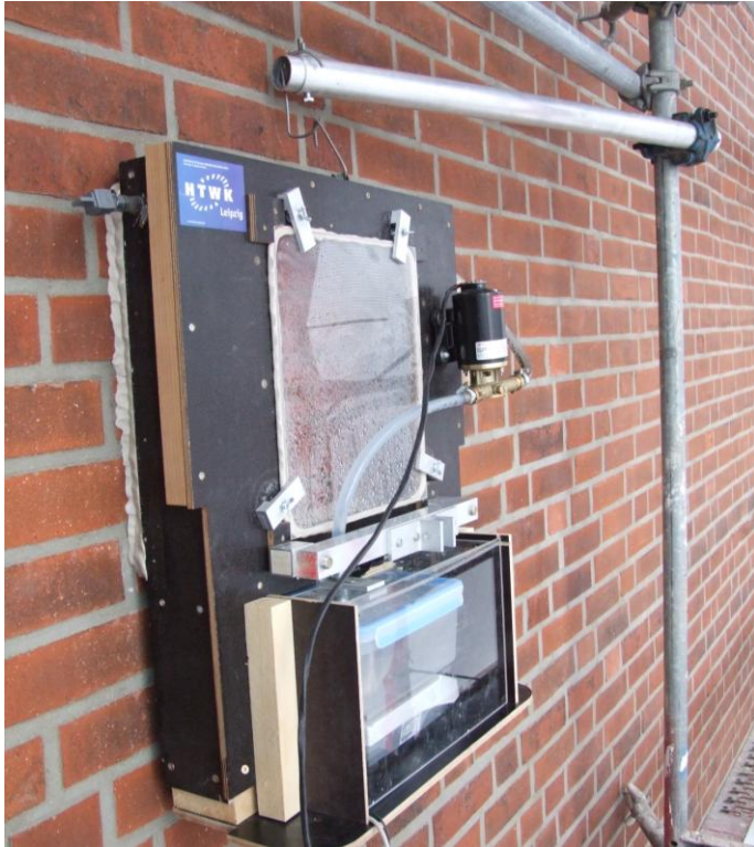
Figure 6. Prototype of developed „Water-Absorption-Measurement” instrument at a historical fair-faced masonry façade.
