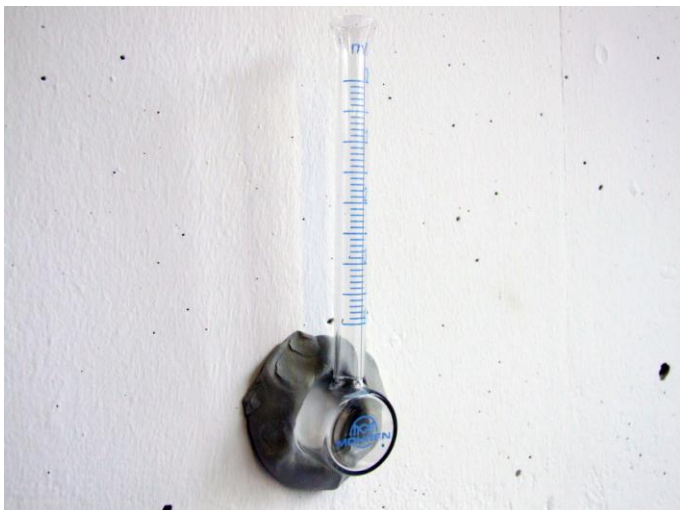
Figure 2. Vertical application of Rilem test method no. 11.4 RILEM tube is fixed on wall.
