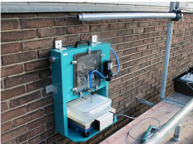
Figure 12. Further development of „Water-Absorption-Measurement” instrument, ready for series production version, WAM 100 B.
