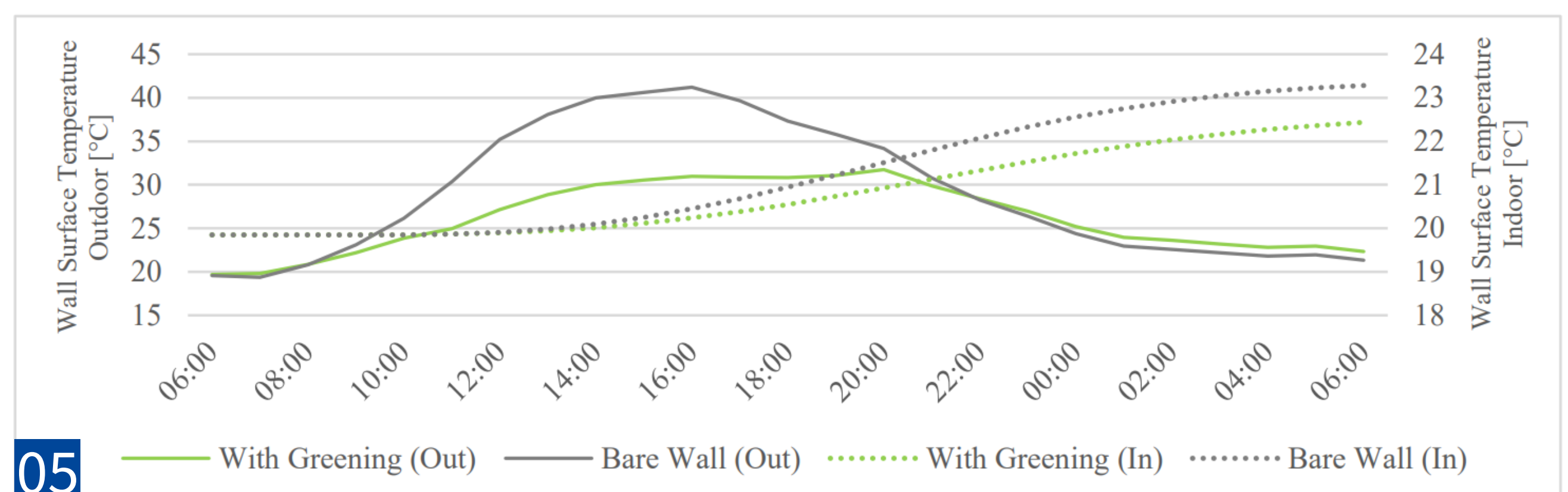
05 Wall surface temperatures with and without greening (Madrid, LAI=1, 2nd floor, south facade)
